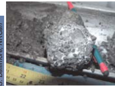
Hydrate (white) and pebbles in drill core
